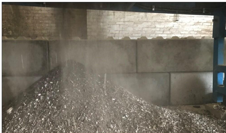
Fig. 2: Trommel fines (image source: www.budget-waste.co.uk )
